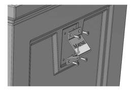
Attach the stainless steel bottle opener with the 4 screws provided. Hand tighten with a screw driver, do not use a power drill.
