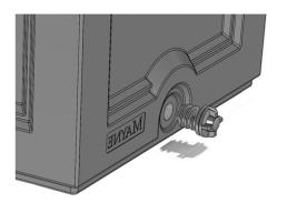
When not in use, partially unscrew the drain plug to let out excess water.
