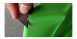
2) Use RAZOR BLADE to remove residual plastic from scape or gauge to try and eliminate any excess.
