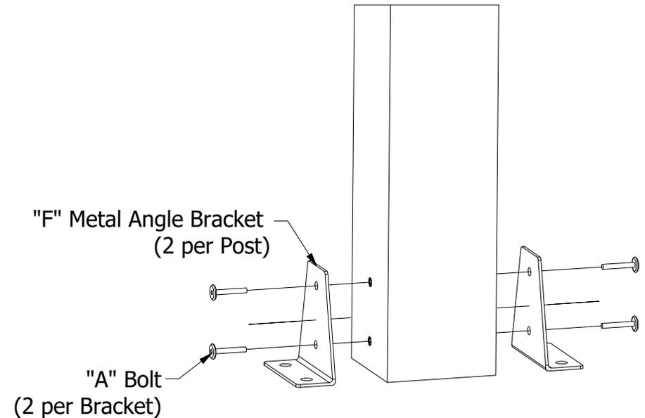
**3)** Attach (2) "F" Metal Angle Brackets to the Bottom of Each Post using (2) "A" Bolts as Shown. Holes in the Brackets will Align with Holes in the Posts.
