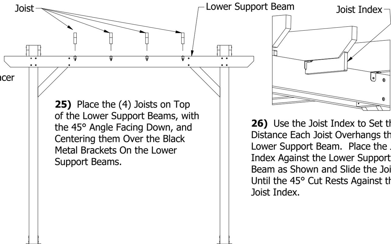
**25)** Place the (4) Joists on Top of the Lower Support Beams, with the 45° Angle Facing Down, and Centering them Over the Black Metal Brackets On the Lower Support Beams.
