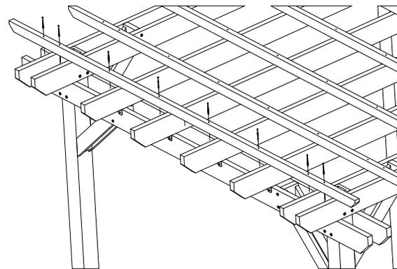
**32)** Secure Each Remaining Top Slat with (7) "D" Screws.
