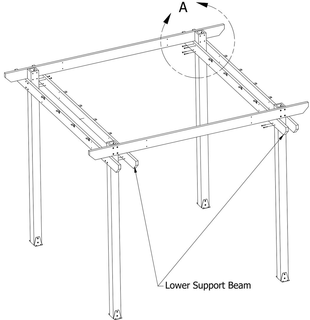
**14)** Attach the Remaining (2) Lower Support Beams Using (16) "B" Bolts, as Shown to the Right and in Detail "A". These Should be Installed on the Opposite Sides of Each Post as the Lower Support Beams Installed Previously, with Metal Brackets Facing Inward.
