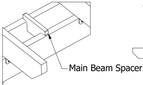
**24)** Place the Main Beam Spacer Between the Lower Support Beams as Shown Above to Maintain the Correct Beam Spacing.
