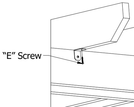
**27)** Secure Each Joist to the Lower Support Beams Using (4) "E" Screws. Center Each Joist Over Each Black Metal Bracket on the Lower Support Beams. This will Set the Center-to-Center Spacing of the Joists. Place a Screw Through the Hole in the Metal Bracket and Secure it Into the Bottom of the Joist.
