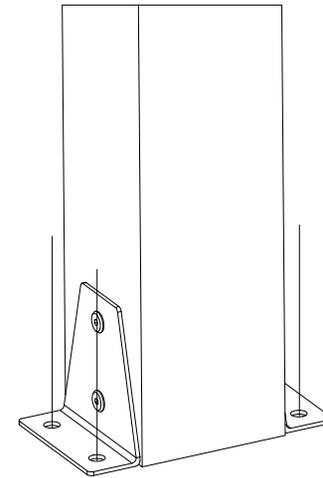
**8)** Once the Arch is in the Desired Location, Support or Add Braces to Hold it Upright While it is Anchored to the Ground. Using Anchors (not included) Appropriate for the Anchoring Surface, Secure the Arch Using (2) Anchors in Each Metal Angle Bracket "F". The Brackets will Support Up to a  $\frac{5}{16}$ " Diameter Anchor.
