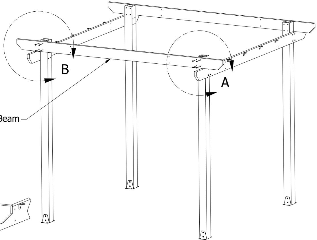
**13)** Lift an Upper Support Beam into Place as Shown and Set on Top of the Lower Support Beams. Secure Both Ends to the Posts Using (8) "B" Bolts, as Shown in Details "A" and "B".
