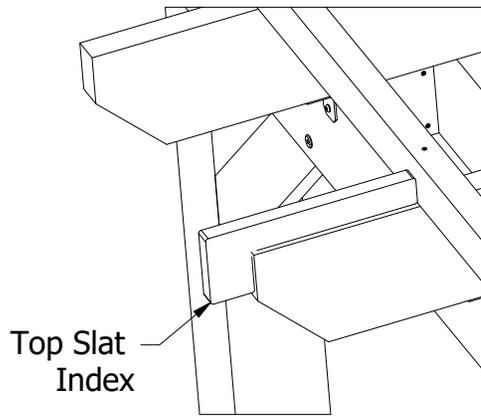
**28)** Place the (7) Top Slats on Top of, and Perpendicular to the Joists and Upper Support Beams, with the 45° Angle Facing Down.
