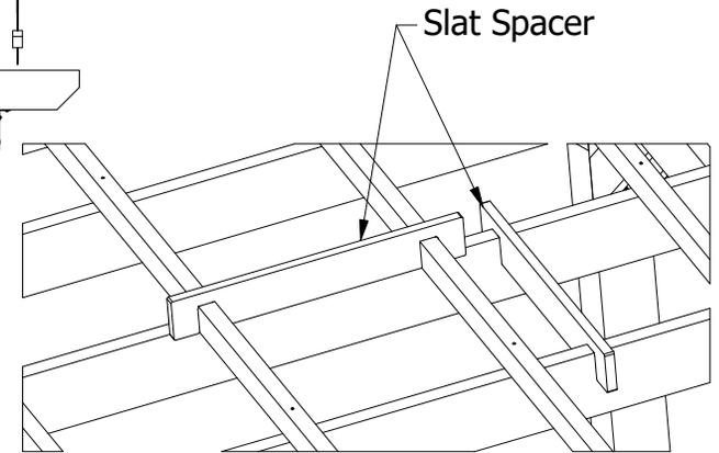
**29)** Use the Top Slat Index to Set the Location of the First Top Slat. Set the Top Slat Index on Top of the Joist as Shown Above, and Adjust the Top Slat Until it Rests Against the Top Slat Index.
